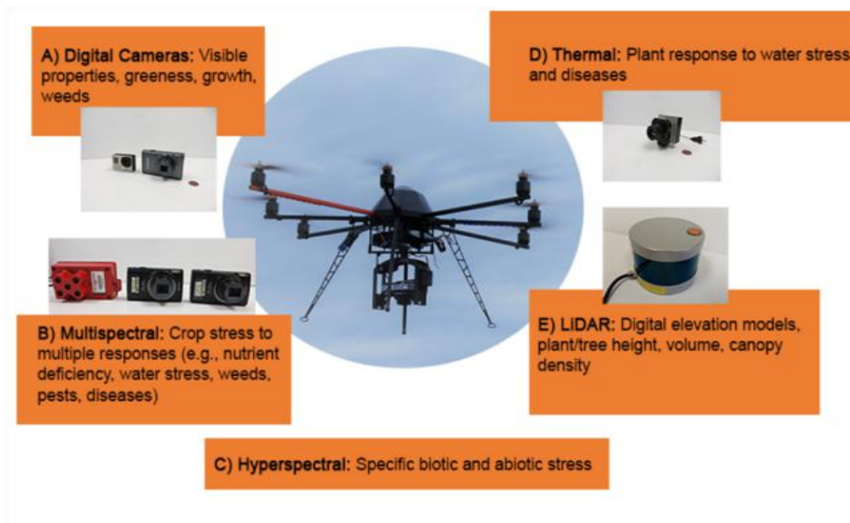
Fig 5.2.1: Realization of agriculture applications using sensors integrated with UAS
